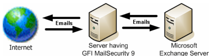
Figure 2 - Installing GFI MailSecurity on a mail gateway/relay server
